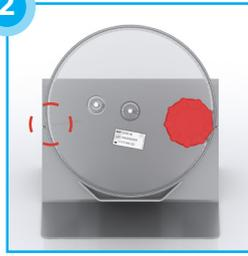
Position CELLdisc™ on the filling accessory with the screw cap either at 105° for right-handed users or 255° for left-handed users (indicated by
