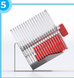
Wait until the liquid is distributed into the individual layers before firmly tightening the screw cap to close it.
