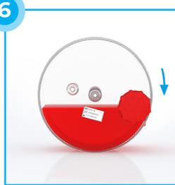
For liquid equilibration, take CELLdisc™ out of the CELLstage, lay it down horizontally and turn it to assure that the medium and all layers are in contact through the central filling channel.
