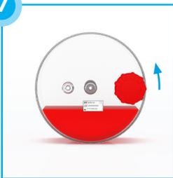
Turn CELLdisc™ as indicated to disconnect mediumflow from the filling channel. Do not rotate CELLdisc™ any further as this could lead to wetting of the filter.
