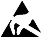
**ELECTROSTATIC DISCHARGE SENSITIVE DEVICE (ESDS):**
