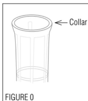
A dual fit adapter is provided to facilitate the ejection of both styles of tip on the 2  $\mu$ l and 10  $\mu$ l models. See section 3.
