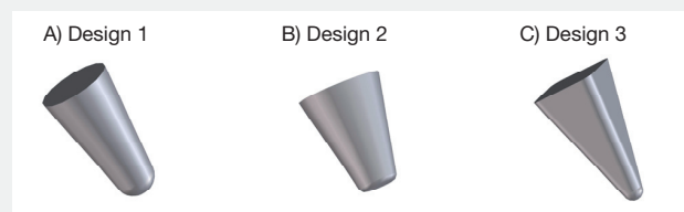
Figure 13: Different Well Geometries. A) Conical well with round bottom B) Conical well with flat bottom C) Blunt cone with a round bottom
