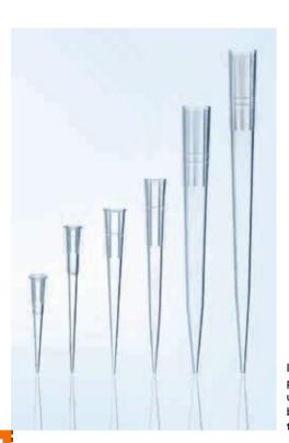
In the case of the Sapphire pipette tips, material usage has been reduced by 20 percent compared to the previous version.
