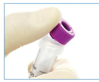
2 The ribbed area around the tube top indicates the cap opening location. Remove the cap by applying gentle pressure on the cap in an upward direction.
