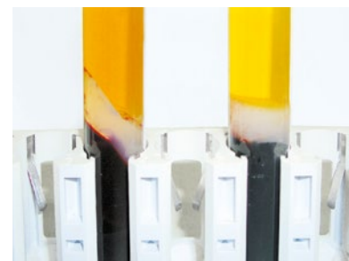
Left: Separator gel tubes centrifuged in a fixed-angle centrifuge
