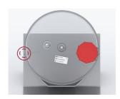
Position CELLdisc on the filling accessory with the screw cap either at 105° for right-handed users or 255° for left-handed users (indicated by ©).
