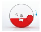
For liquid equilibration, take CELLdisc out of the CELLstage, lay it down horizontally. Turn it to assure that the medium and all layers are in contact through the connecting channel.
