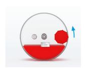
Turn CELLdisc as indicated to disconnect mediumflow from the filling channel. Do not rotate CELLdisc any further as this could lead to wetting of the filter.
