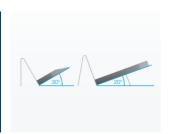
CELLstage guarantees an exact filling angle of 30° for CD4-CD24 (878072) and 20° for CD40 (878073).
