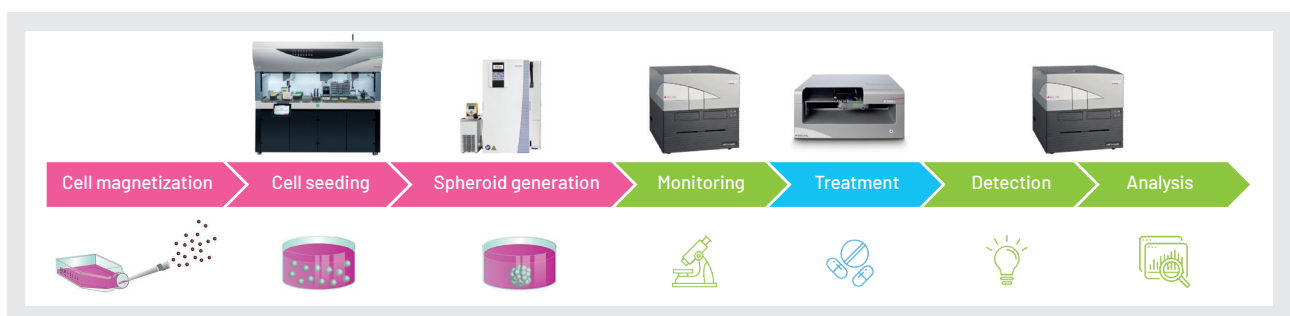
Figure 2: Schematic overview illustrating a drug screening workflow using the Fluent Automation Workstation, D300e Digital Dispenser and Spark Cyto multimode reader.
