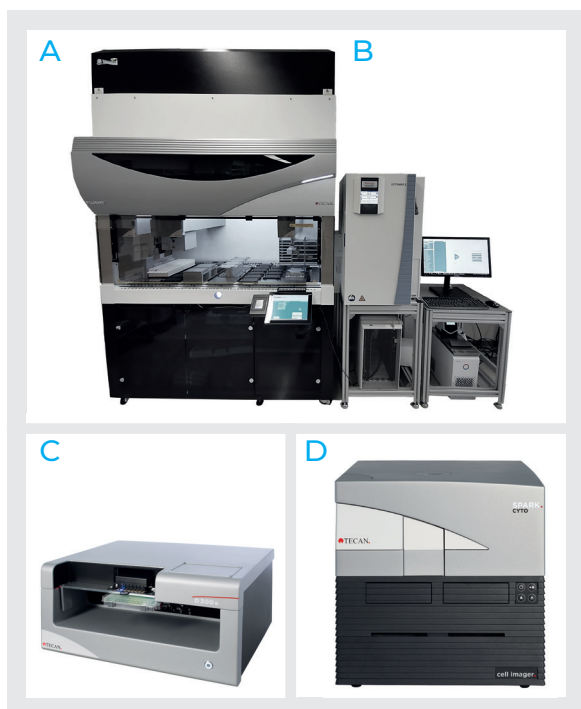
Figure 3: A Fluor Automation Workstation (A) was integrated with a Cytomat 2 C450-LiN Automated Incubator (B) to automate the preparation and storage of the spheroid microplate. The D300e Digital Dispenser (C) was used for drug dispensing, while imaging and measurement of the chemiluminescent signal were performed with a Spark Cyto 600 (D).
