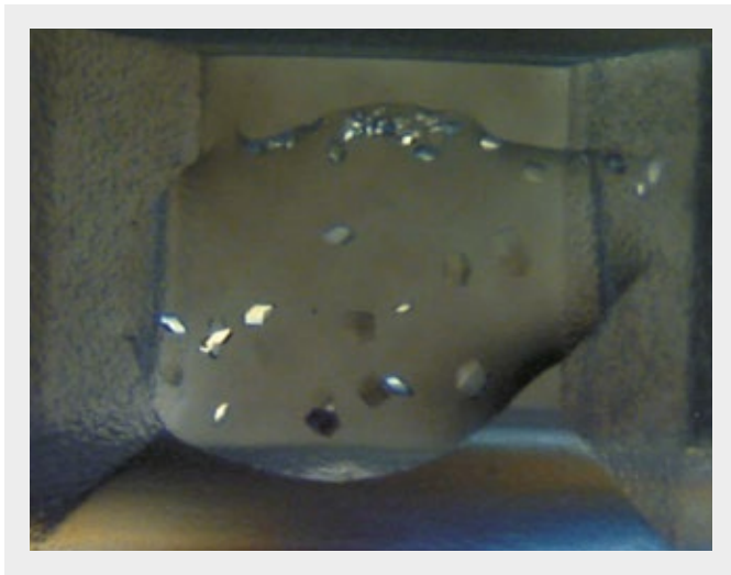
Figure 6: Microscopic detection of protein crystals with polarised light through AMPLIseal
