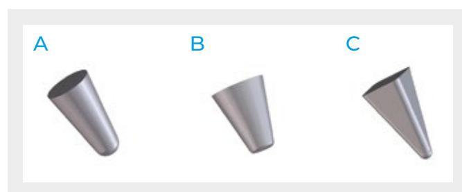
Figure 12: Different well geometries. A) Design 1 – Conical well with round bottom B) Design 2 – Conical well with flat bottom C) Design 3 – Blunt cone with a round bottom.
