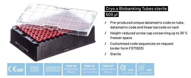
Height: 33.3 mm, Total rack height: 36.2 mm, Ø: 8.8 mm, Barcode type: datamatrix code, Raw material: PP, Working volume: ≤580 μl, Cap design: screw cap, Sterile: +
