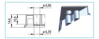
**Figure 3:** Well profile: 96 well F-bottom / ST, polystyrene Total volume: 382 µl Working volume: 25 – 340 µl Growth area: 32 mm<sup>2</sup>
