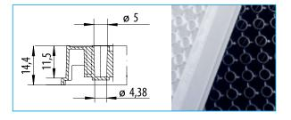
Figure 5: Well profile: 96 well Half Area Total volume: 199 µl Working volume: 15-175 µl Growth area: 15 mm<sup>2</sup>
