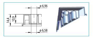
Figure 4: Well profile: 96 well F-bottom / chimney well, polystyrene Total volume: 392 µl Working volume: 25 – 340 µl Growth area: 34 mm<sup>2</sup>
