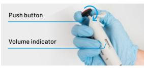
Set the volume by turning the push button. To obtain maximum accuracy, proceed as follows:
