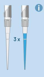
This simple "prewetting-procedure" prevents that your first few dispenses deliver less volume due to evaporation effects. Another risk that is accompanied by evaporation is an increase in vapour pressure so that liquid is forced outside the tip which can result in droplet formation at the tip end. In order to reduce user-related pipetting errors (when using an air-displacement pipette), pipette in between 35 and 100 % of the nominal volume range.
