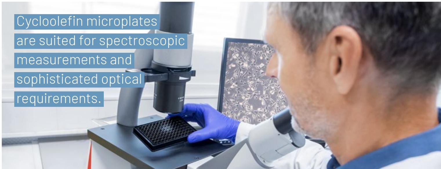
**Cycloolefin** is the material of choice for microplates with special requirement profiles. A low level of autofluorescence, along with exceptional transparency in lower UV wavelengths, enables cycloolefin microplates to be utilised for spectroscopic measurements in the UV range (UV-Star® microplates). The chemical stability of cycloolefin to polar solvents like DMSO, together with an extraordinarily low vapour diffusion rate, render the base material
