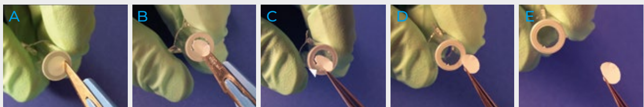
Figure 3: For the detachment of the capillary pore membrane from the insert housing a scalpel is plunged into the membrane adjacent to the insert housing (A). The membrane is cut out moving the scalpel alongside the inner edge of the housing (B), thereby leaving a small segment attached to the membrane (arrowhead in C). Finally, using tweezers, the membrane is torn off the housing (C-E). The membrane is now ready for further processing such as mounting onto a microscopy slide, sectioning or other applications.
