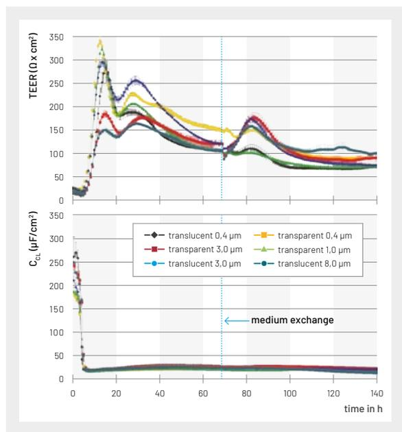
**Figure 3:** TEER and  $C_{\text{CL}}$  recordings on MDCK-II cells cultivated on ThinCert® cell culture inserts with different pore sizes. Increasing transepithelial electric resistance values (TEER) correlate with a decreasing capacitance ( $C_{\text{CL}}$ ) of the cell layer. After 60 hours the TEER values level out at 100–160  $\Omega \times \text{cm}^2$ , thus indicating confluence and formation of a tight cell layer. The dashed line indicates the time point of medium exchange.
