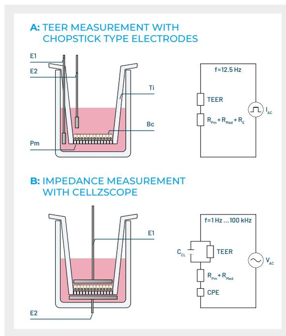
**Figure 2: TEER and impedance measurements with chopstick-type electrodes and the cellZscope system.**
