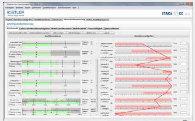
Figure 3: Result of operating point optimisation with Stasa QC for Greiner Bio-One roller bottles. The graphic display of the relationships between process parameter settings (right) and quality features (left) provide an overview of the process (red: optimum operating point and process window) and at the same time enables interactive simulation of the process. The values for the process setting parameters have been obscured in order to protect process know-how (Photo: Stasa)
