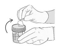
**NOTE**: In a <u>closed</u> beaker, the minimum fill level should be 20ml when sampling only one tube; and 40ml when sampling more than one tube. The maximum fill level should be 100ml.
