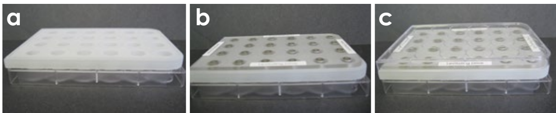
Fig. 3: Take a cell-repellent 24-well plate, place the custom lid atop the cell-repellent 24-well plate, (a) place a 24-well levitating drive atop the custom lid, (b) and place the regular lid atop the 24-well levitating drive to levitate the cells (c).
