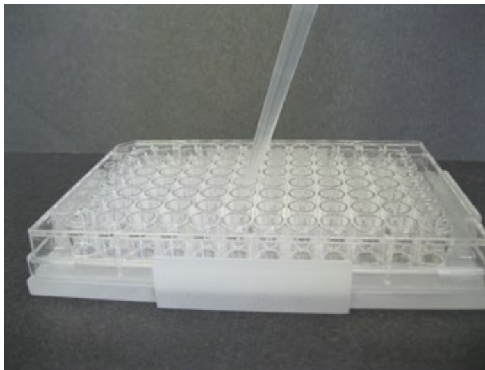
Fig. 4: Use the 96-well holding drive to hold 3D cultures as you add and remove liquids
