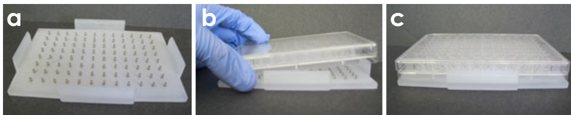
Fig. 3: Take a 96-well spheroid drive (a) and place a cell-repellent 96-well plate (b) atop the 96-well spheroid drive to print the cells into a spheroid (c).
